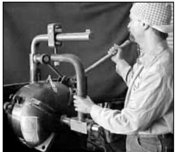
FIGURE No. 6 WRONG Operating Position!
